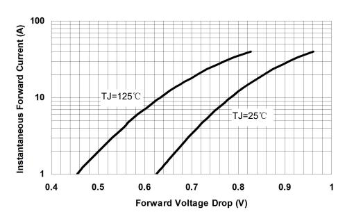
Fig.3-Typical Instantaneous Forward Voltage Characteristics
