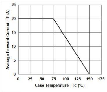
Fig.4 Max. Allowable Case Temperature Vs. **Average Forward Current (Per Leg)**
